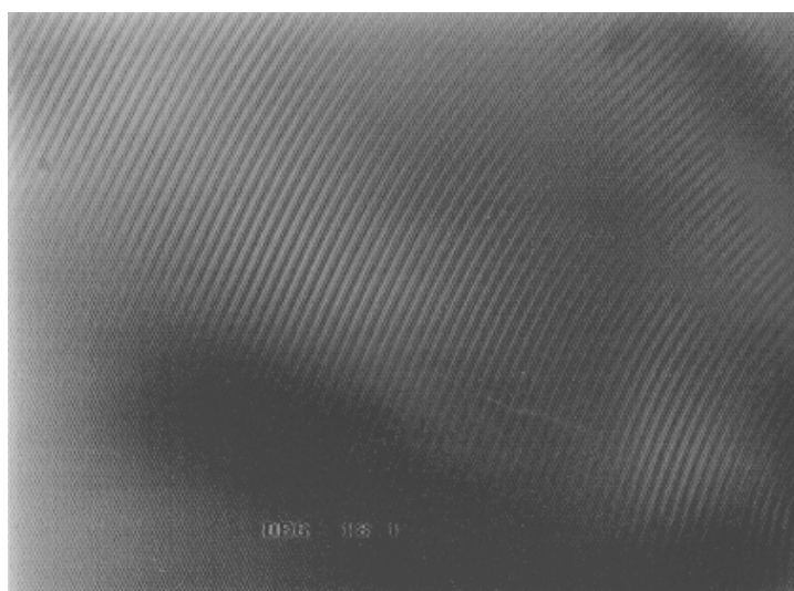
Figure 12 Optical micrograph between crossed polarizers of a 10% w/w solution of L,L-PIAA in \text{CHCl}_3 .
