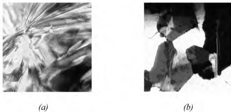
Figure 5.3 Typical textures observed with TOPM for clip molecules 2 and 3 . (a) Polychromatic texture. (b) Platelet/mosaic texture.
