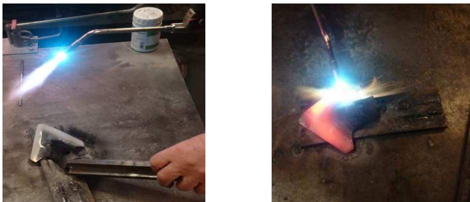
Figure 2. The layer-build-up of alloy powder by means of hot metal powder spray fusing.
