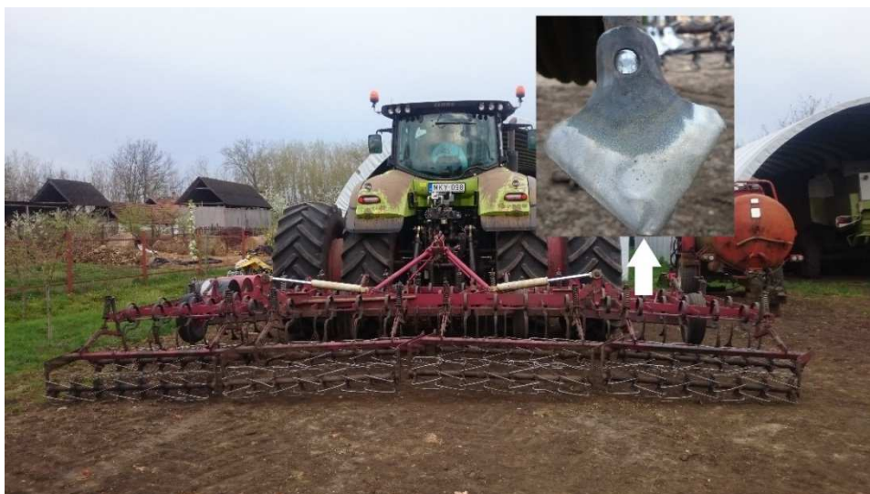
Figure 6. Agricultural machine equipped with cultivator tines.
