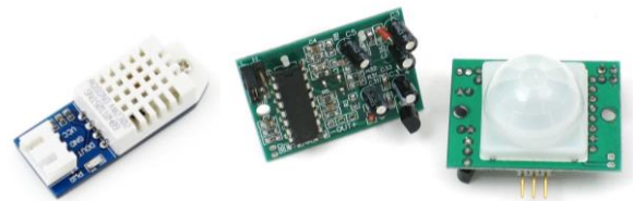
4.ábra Smart Mirror sensors - DHT-22 & PIR [12][13]
