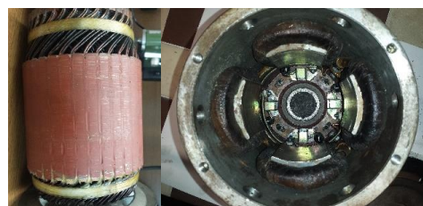
Fig. 2. The rotor (left) and stator (right) of the electric motor.
