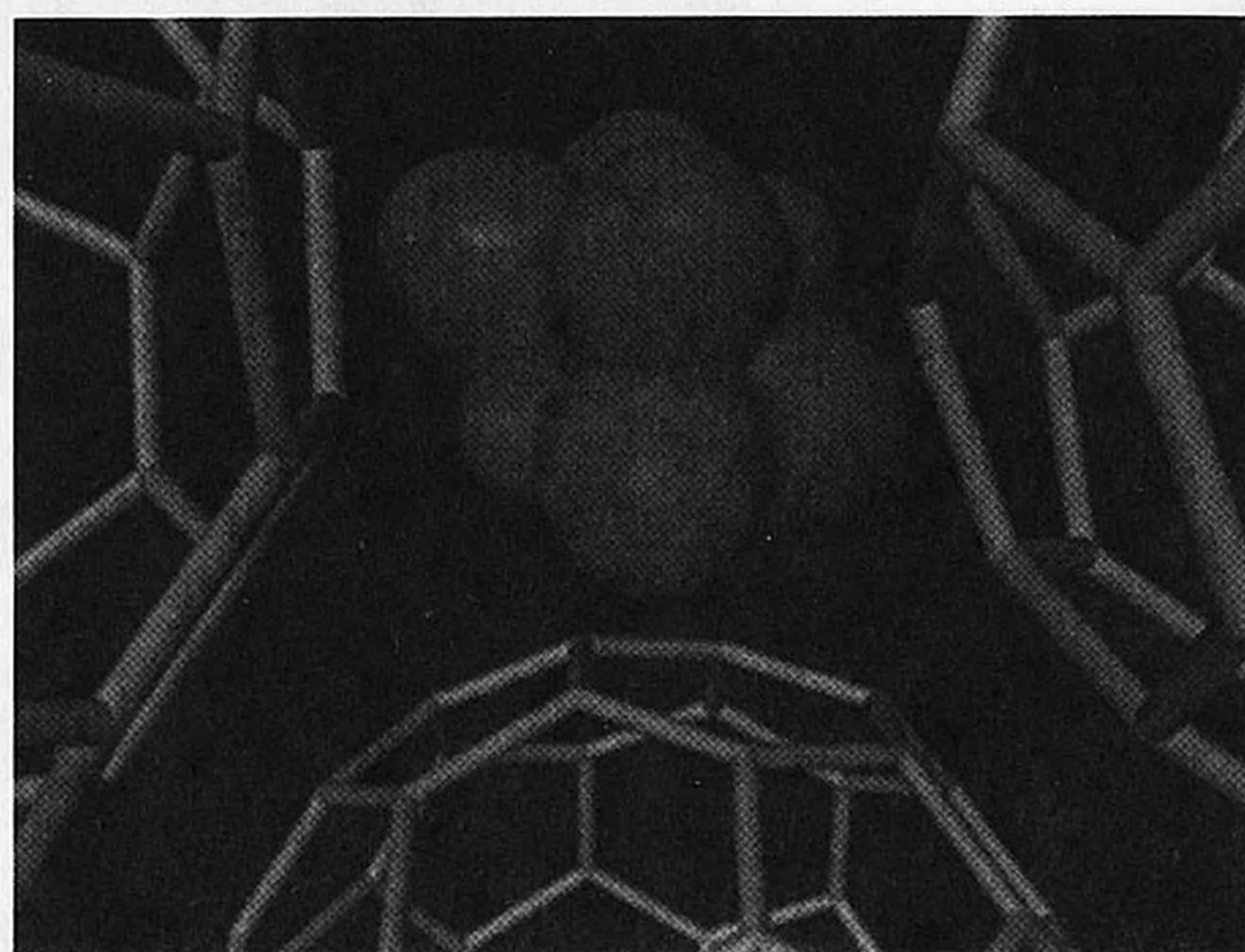
FIG. 3. A 3D equipotential cut ( 85 \text{ cm}^{-1} above the global minima) through the 5D potential energy surface is shown, indicating the position of the center of mass of CO for an optimized CO orientation, with all C_{60} molecules in the major orientation. This potential has six global and two local minima along the cube diagonals.
