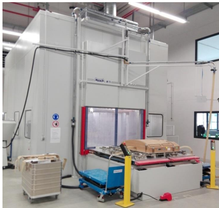
Fig. 2 MAKKA M7t type CNC driven milling machine [1]
