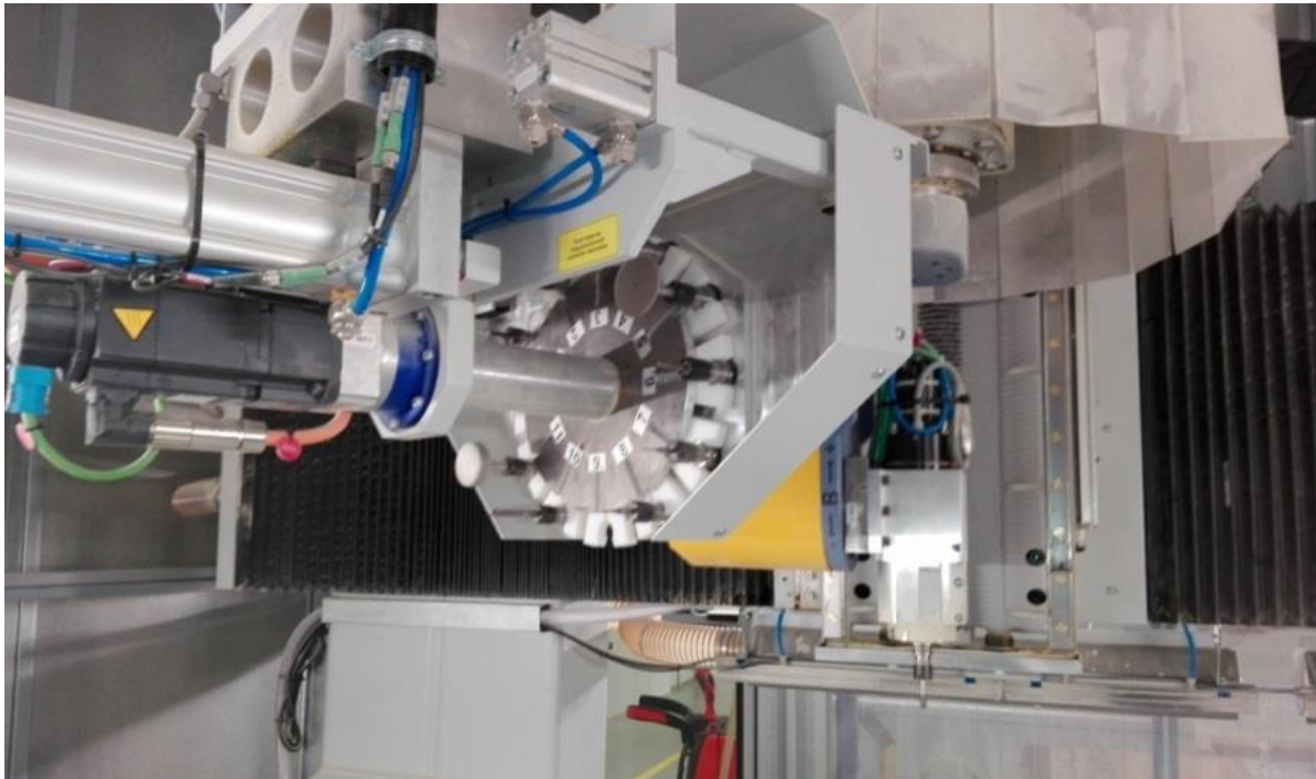
Fig. 3 Main spindle and the tool storage with 12 tool places
