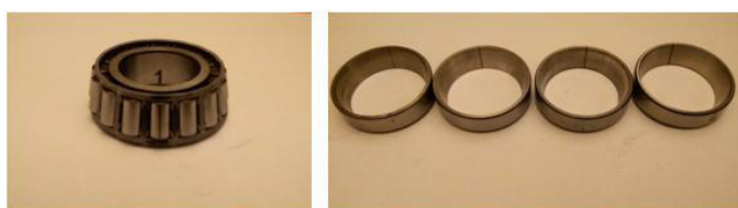
Fig. 5 Roller fault and OR faults in the experiment
