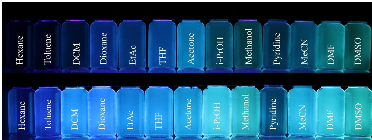
Figure 3. Visible fluorescence of ACAIN (top) and ACAIN-propanethiol adduct (bottom) in solvents in order of increasing polarity excited at \lambda=365 nm. All solutions have the same concentration: 25.4 \mu M
