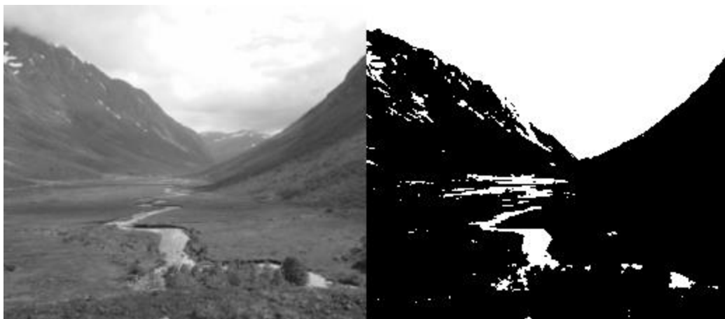
Figure 3-4 An arbitrary image (left), along with the resulting image from thresholding (right) [43].
