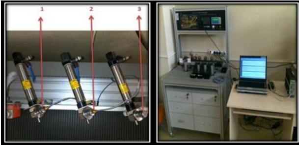
Fig 4. Separator pneumatic test and separation station and an experimental setup for measuring the acceleration (1).
