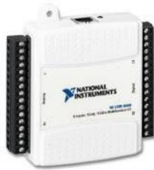
Figure 3, NI USB-6009 USB Student Data Acquisition Kit, NI USB-6009 Student Kit for USB (Figure 3) is a perfect cost effective true multifunction DAQ capability device, provides 48 kS/s at a resolution of 14 bits, eight single-ended (four differential) analogue inputs; also provide two true analog outputs and 12 digital I/O lines (5 V TTL/CMOS).
