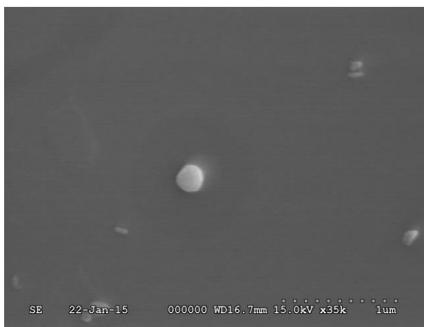
Figure 4. SEM image of a purified elemental selenium nanosphere (Hitachi SEM)
