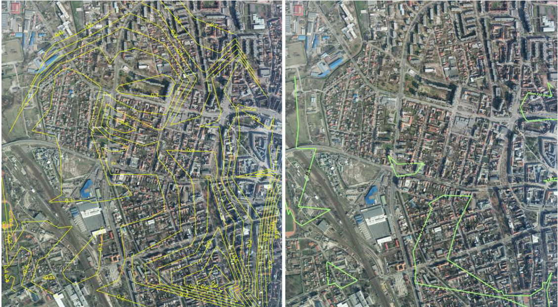
Figure 1. Horizontal deviations in the DEM (yellow marking) and in the terrain model created by photogrammetrical assessment (green marking) in the Nyíregyháza area depicted with isolines at 10 cm intervals. (own edition)
