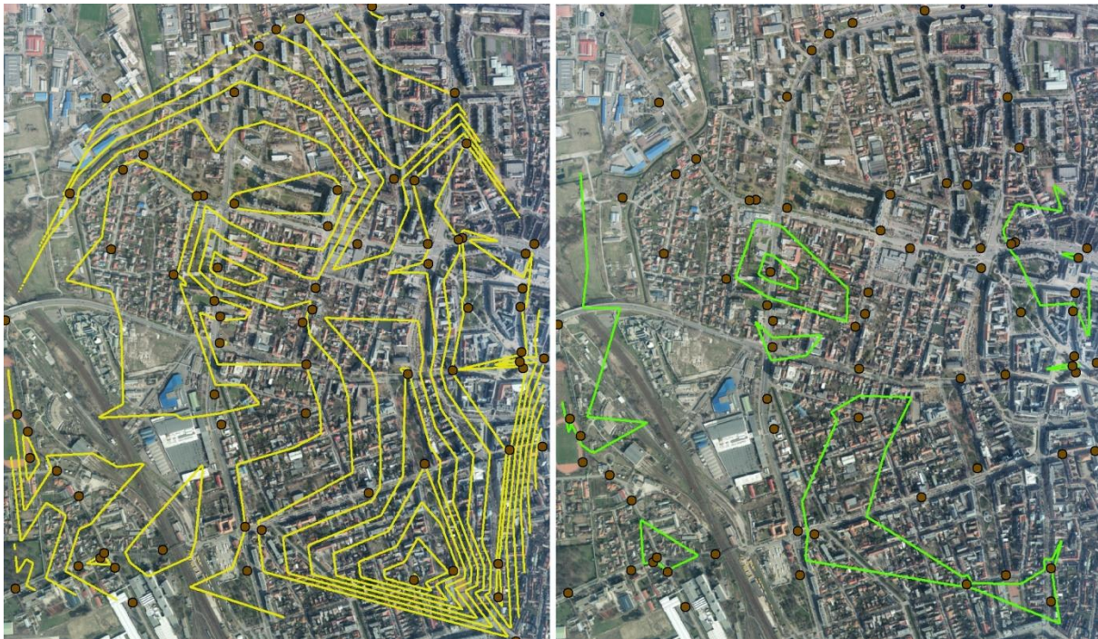
Fig. 5 Horizontal differences in the DSZM (yellow), and on the digital terrain model prepared with photogrammetric interpretation (green) in Nyíregyháza
