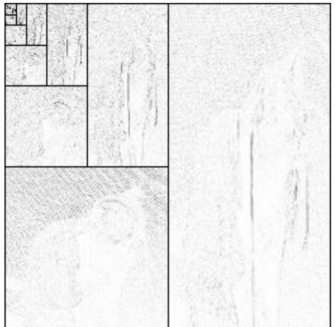
Figure 6 Detail coefficients of the wavelet transform of Figure 5 image.
