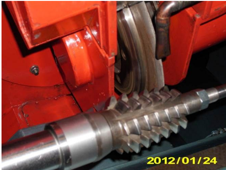
Figure 7. The hob backward grinding could be seen on this figure (DifiCAD Engineering Office Ltd.)
