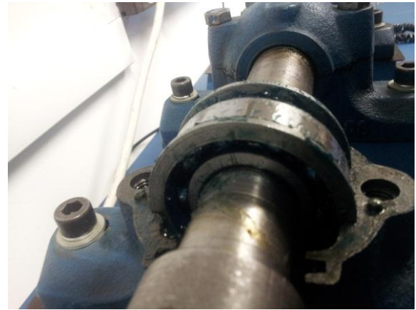
Fig. 5. Bearing test rig for validation
