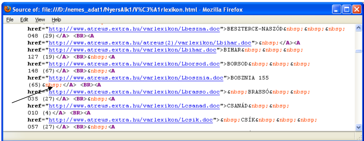
Fig. 4. The source of the web page presented in Fig. 2 when opened in a text editor. The text is loaded with normal and Non-breaking Spaces. Arrow points to the extra Non-breaking Space following county Bosnia, inclosed in the Anchor tag (<A></A>).
