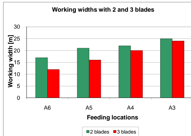
Fig.7 The obtained working widths by using two and three blades
