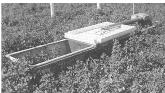
Figure 2: Automated field chamber for measurement of gas fluxes from soil
