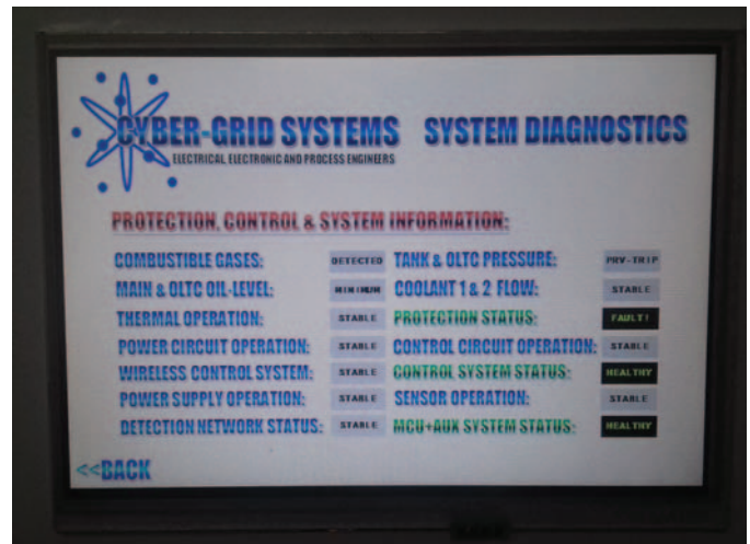
Figure 9: ACM System with local diagnostics
