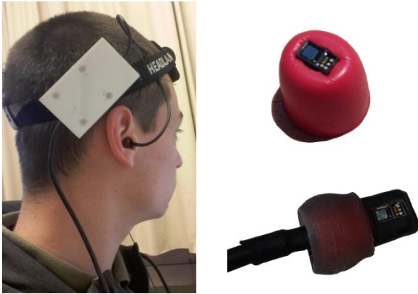
Figure 2 a) In-ear PPG system prototype attached to the head. b) Axially oriented optical sensor with off-the-shelf foam earbud adapter. c) Radially oriented optical sensor with off-the-shelf rubber earbud adapter.
