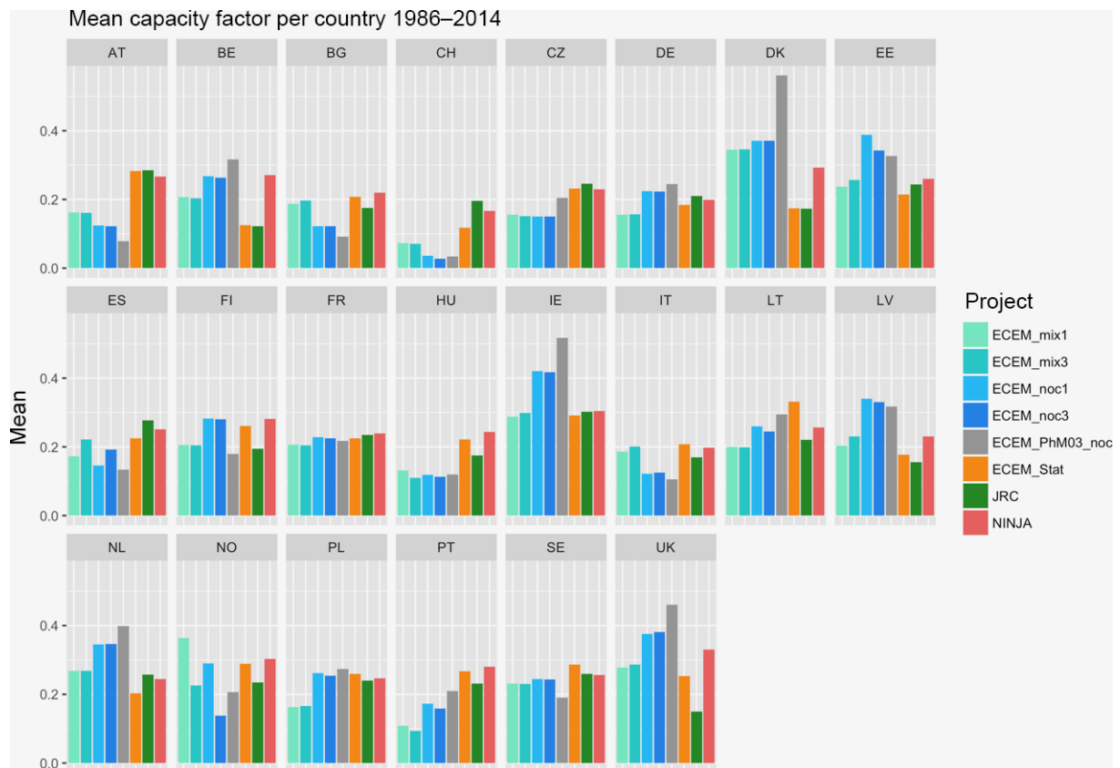
Figure 6. Country-average wind power capacity factor for C3S ECEM wind power models, and JRC (EMHIRES, green) and Ninja (salmon) datasets. In model mix1 and noc1 the known installed capacities from the WindPower database were used; in mix1 a mix of bias-adjusted 100 m wind speed were used (i.e. bias-adjusted over land and non-bias-adjusted over the ocean), in model noc1 the original ERA-I extrapolated to 100 m wind speed were used. In PhM03_wbc , the bias-adjusted 100 m wind speed data were applied to a fixed wind turbine type at each 0.5° by 0.5° grid cell. Finally, Stat is the statistical model using the support vector machine approach.
