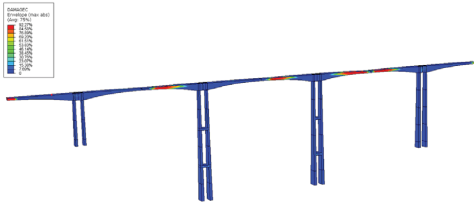
(a) Compressive damage under the 'Best' case excitation
