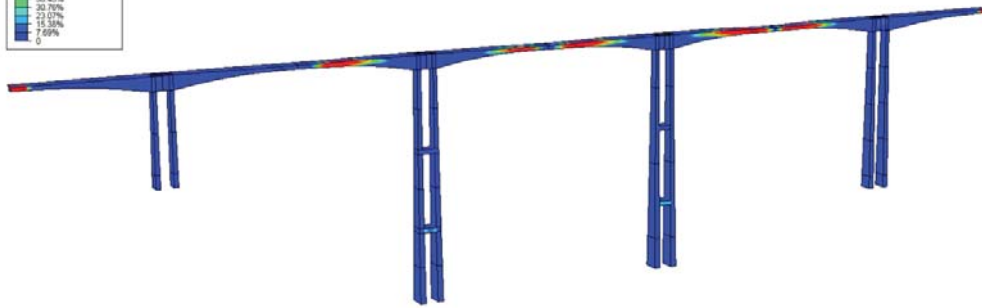
(c) Compressive damage under the 'Worst' case excitation
