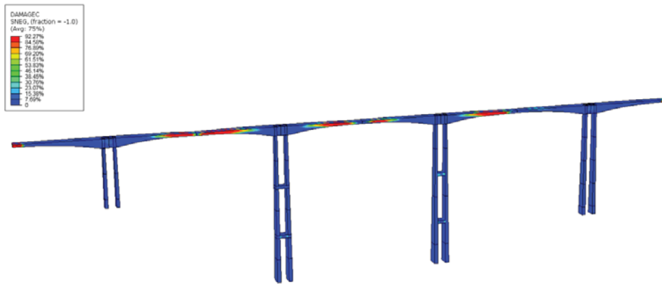
(b) Compressive damage under the SVGM excitation
