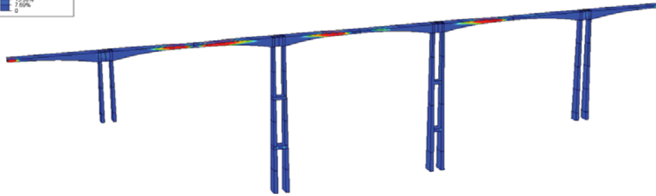
(b) Compressive damage under SVGGM excitation
