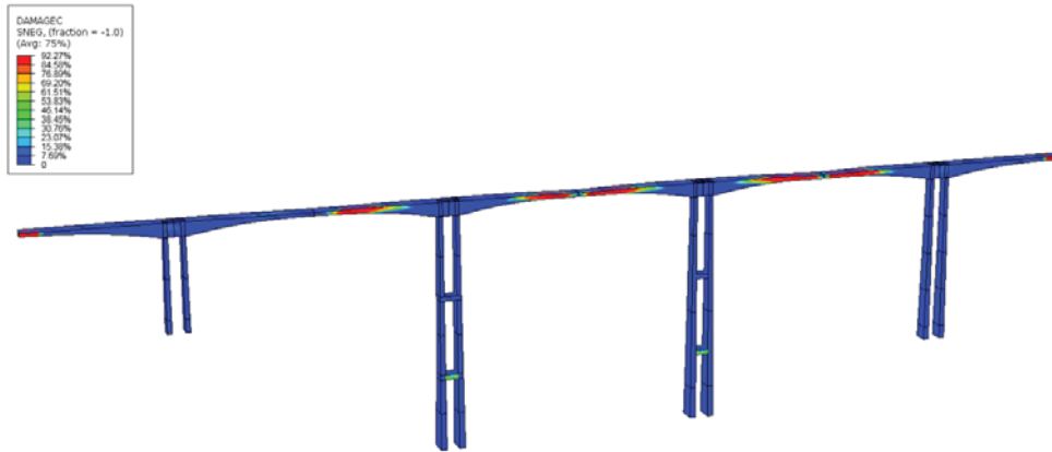
(c) Compressive damage under the 'Worst' case excitation
