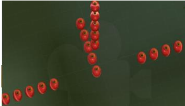
Figure 5. Calibration setup includes picking apples located in different distances in four directions to obtain users’ range of motion.
