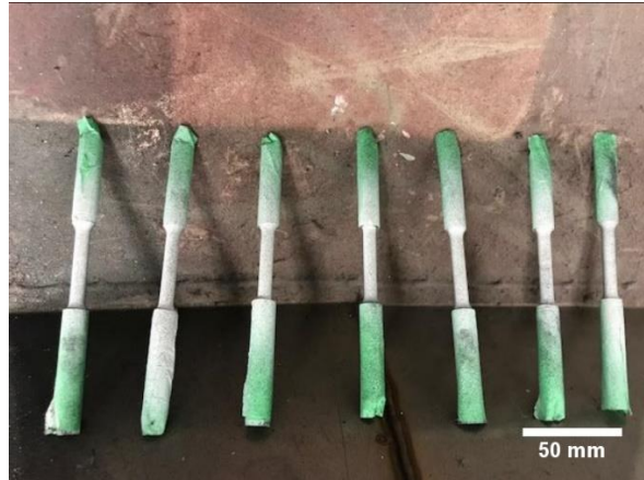
Figure 3.5: Tensile samples after the application of the two layers of painting.
