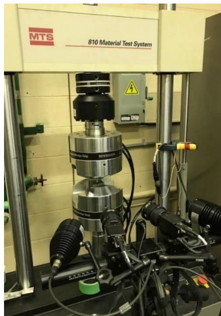
Figure 3.6: Setup of the MTS frame with the cameras for tensile tests using the DIC technique.
