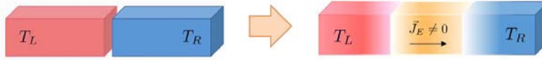
Figure 1. At t = 0 , both systems are isolated and independently at equilibrium. Evolving forward in time from t = 0 , a spatially homogeneous non-equilibrium steady state develops in the middle region, carrying an energy current J_E .
