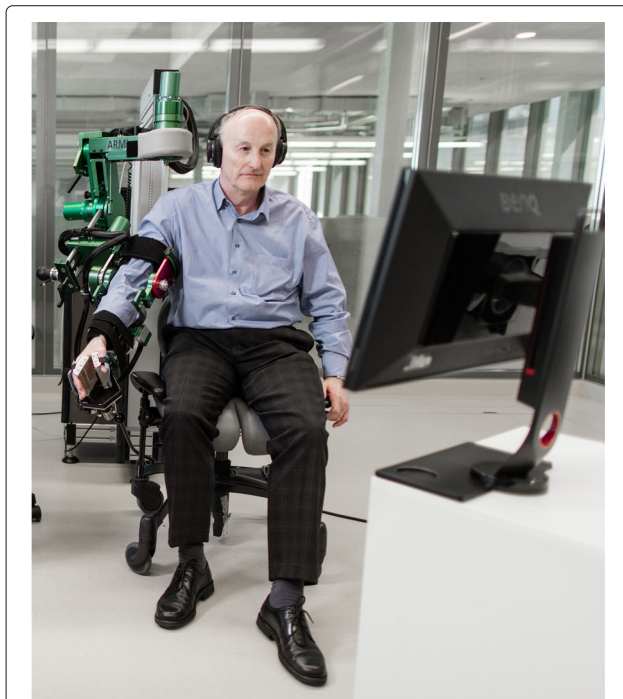
Fig. 1 ARMin arm rehabilitation robot. Additionally for this study, a keyboard was placed close to the participant's left hand so that the space bar could be used as input device
