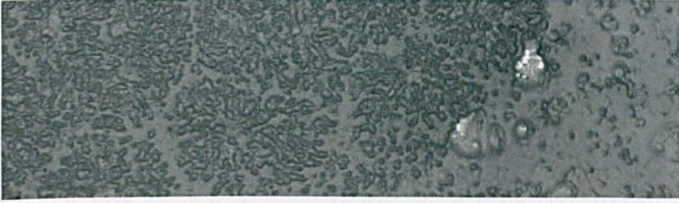
Figure 7.51 Interferometry scanning of a mixture of crude oil and heptane adsorption through brine into silicate surface.
