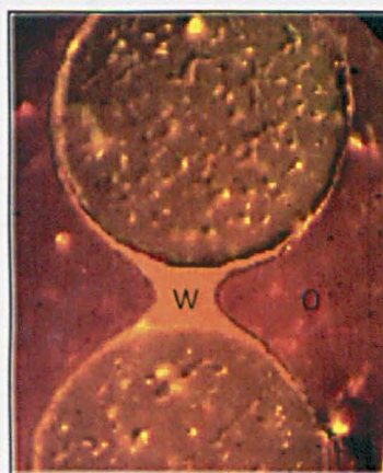
Figure 5.2 After micromodel cleaning, pore throats are occupied by water which indicates the water-wetting state of micromodel. (Yellow=water, Brown=oil).
