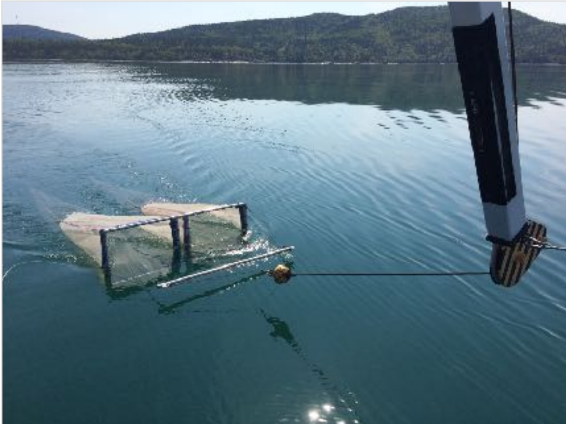
Figure 1: Paired neuston nets and boom. Photo: Mark Vinson, USGS 2014
