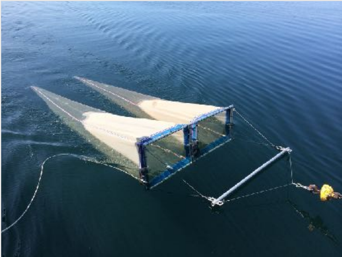
Figure 2: Paired neuston nets. Photo: Mark Vinson, USGS 2014
