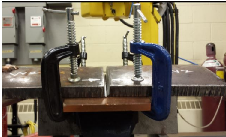
Figure 7.1: Welding fixture setting.
