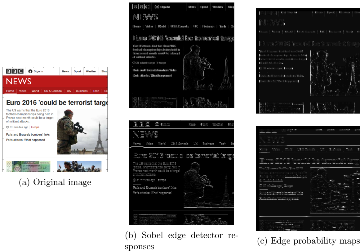
Figure 3.8: Comparison of original image, Sobel edge detector responses, and a map of the probability of a locally significant edge.
