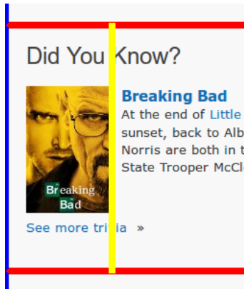
(a) A coincidental alignment of edges within text (the letter “K”) and the edge of a thumbnail, detected as a spurious low-level edge. The underlying web page is the IMDB home page.
