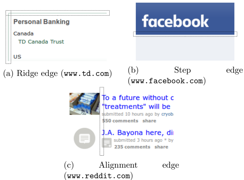
Figure 3.2: Types of edges commonly found in web pages, illustrated with examples from real web pages.
