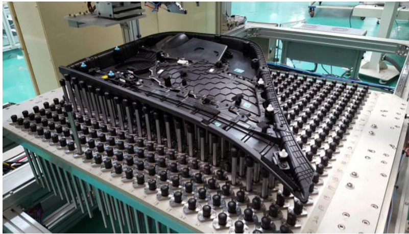
Figure 1-4. Transformable assembly jig (SEOYON E-HWA corp.)
