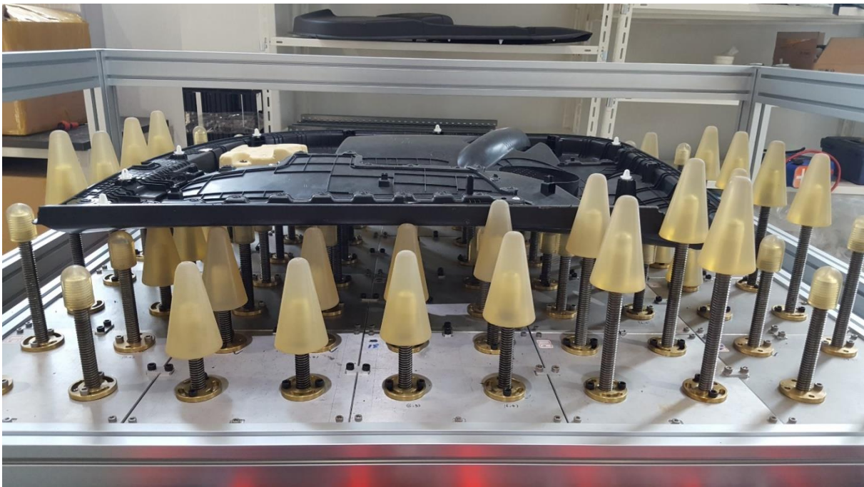
Figure 4-6. Typical loading posture of assembly part
