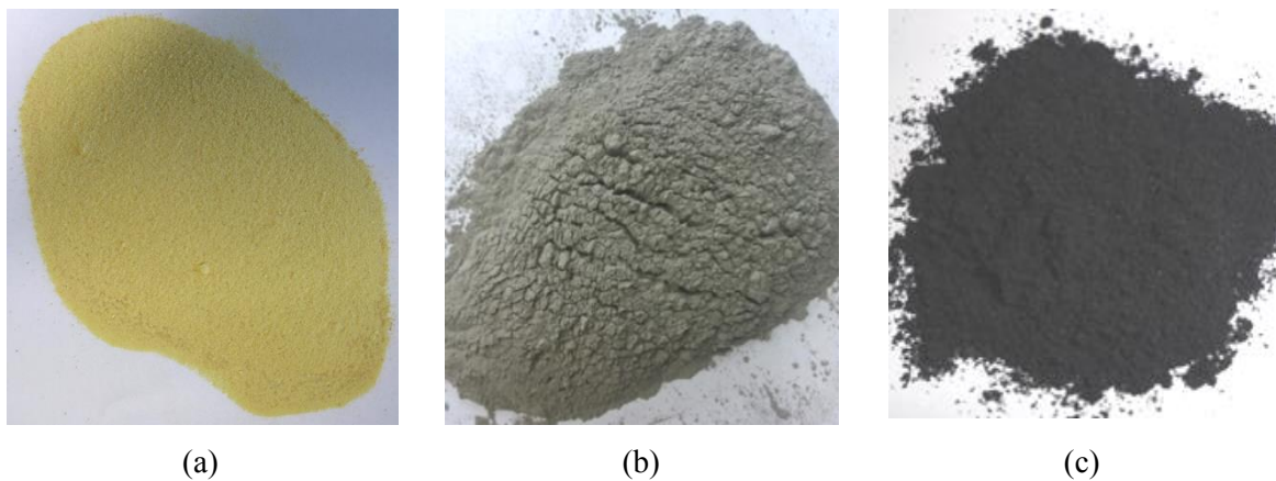
Figure 3-1: Raw materials: (a) modified sulfur, (b) fly ash, and (c) rubber powder.
