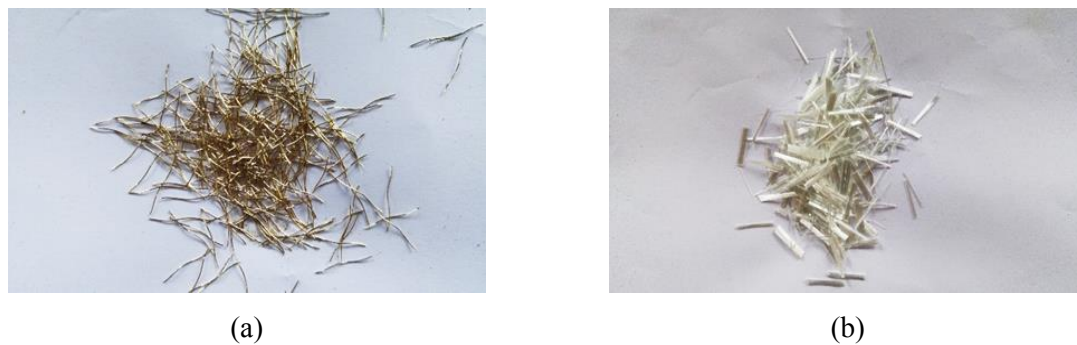
Figure 5-1: Micro fibers: (a) steel fiber, and (b) ECR glass fiber.
