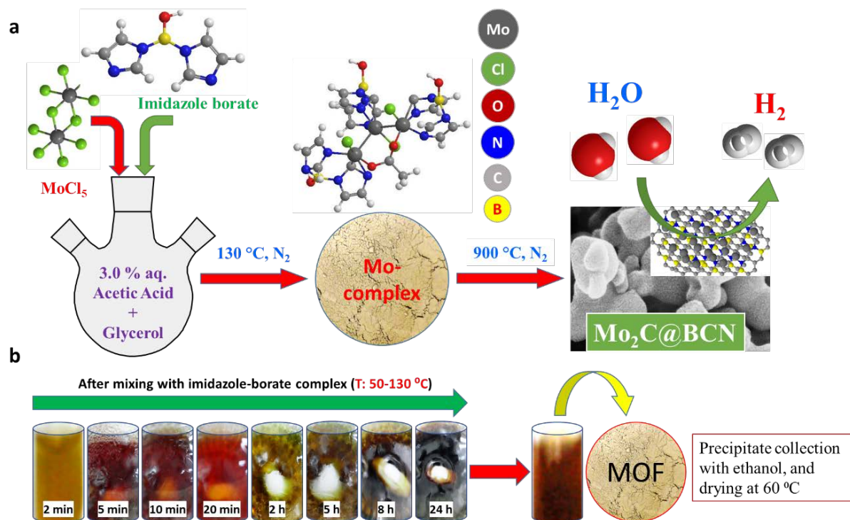
Figure 2.1. (a) Schematic illustration for preparation of BCN-encaged different phases of molybdenum carbide and evolution of color during the synthesis of Mo-Im-Borate complex.
