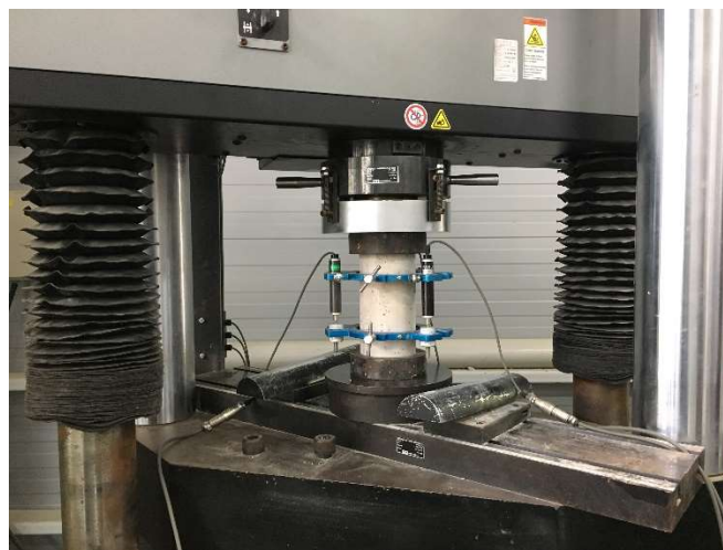
Figure 16. Compressive strength test on the concrete specimen
