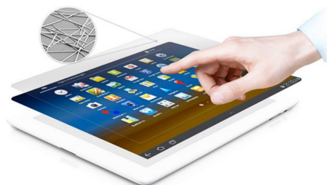
Figure 1.16. The illustration of commercial touch screen with AgNW-based transparent electrodes. (Cambrios Technologies Corp., http://www.cambrios.com/ , accessed: May 2018.)
