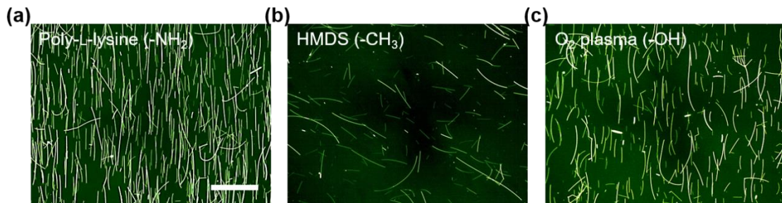
Figure 5.5. Dark-field optical micrographs of the aligned AgNW networks coated on substrates modified with different types of functional groups; (a) PLL (-NH 2 ), (b) hexamethyldisilazane (HMDS) (-CH 3 ), and (c) O 2 plasma (-OH). During the bar-coating assembly, #2 bar, 3 μl of volume, and 10 mm s -1 of coating speed were used in all experiments. The scale bar is 40 μm.
