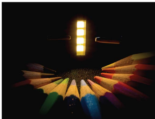
Figure. 1.14. The photograph of white OLEDs with angular color stability incorporated with AgNW-based transparent electrodes. (Gaynor et al. Adv. Mater. 2013 , 25 , 4006) 2
