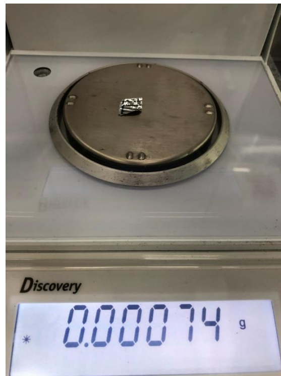
Figure 4.12. A photograph of ultralight PSC device put on an electric scale, indicating extremely light weight.
