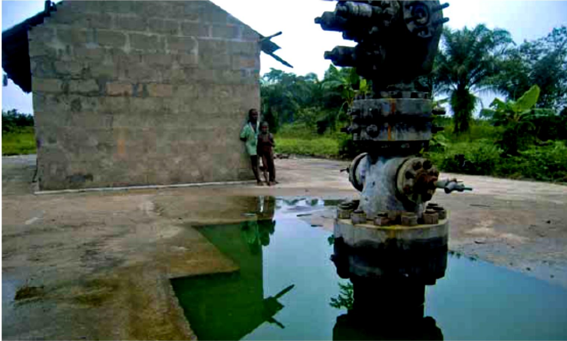
Figure 2.4: A house constructed on a well pad (Yorla 9, Khana LGA)
