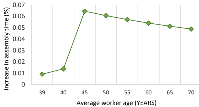
Figure 5. Trend in increase of percentage of assembly time for workers under different ages.
