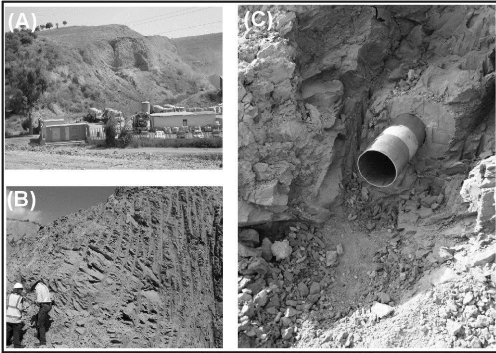
Figure. 2. Sampling site: (A) The Misterbianco quarry. (B) In outcrop well developed fissures in the clays with an apparent dip out of the face (C) Horizontal tube sampling of C1.
