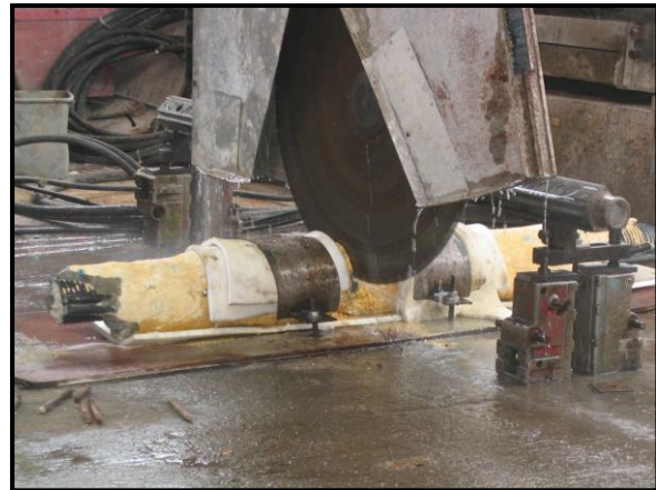
Plate 2 - Preliminary soil nail being saw cut
