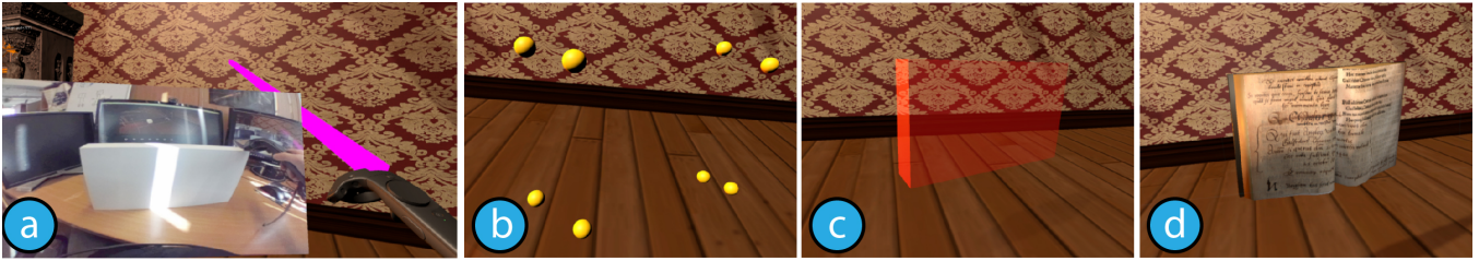
Figure 3: Above, the sequence of actions necessary to identify a physical object and substitute it with a mismatching virtual object, as shown from the HMD-based interface. In (a), the white box is chosen for substitution; successively the user draws eight vertices around the physical corners of the box through the tracked Vive controller (b); a box is fitted within these eight vertices (c); finally, the chosen object is fitted within its bounds (d).
