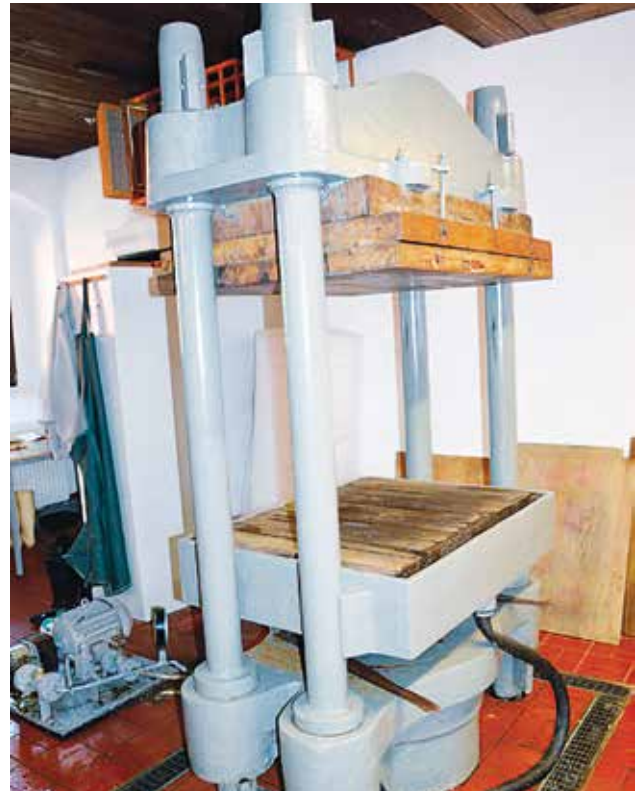
Photo 56. Paper laying equipment – the press Photo by A. Fortuna-Marek
