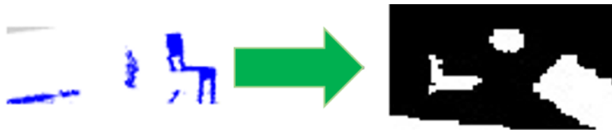
Figure 3.6 Map of 3-D point cloud (left) as it corresponds to a 2-D grid map (right). The white regions of the map have points projected onto the floor and the black regions are labeled as background.
