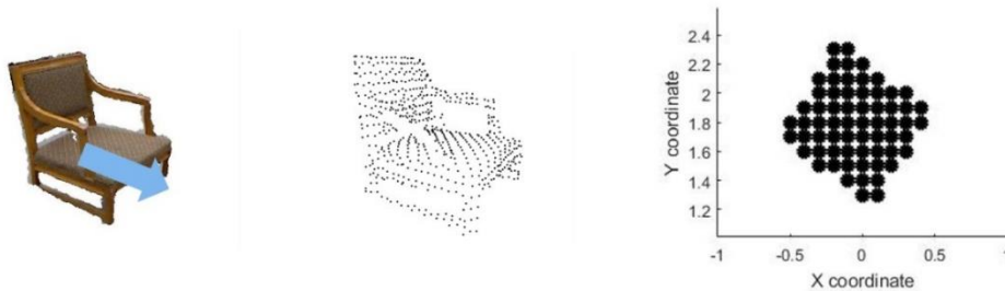
Figure 3. An example of using entity model to describe a chair. LEFT: the chair sample (The arrow illustrates its direction); MIDDLE: the 3-D point cloud of the chair; RIGHT: the 2-D point cluster \rho . The direction angle is 4\pi/7 rad (or 315^\circ ). The entity model e = \{“chair”, \rho, 7/4\pi\} .
