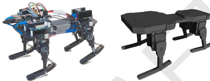
Fig. 1: On the left, the quadruped Tigrillo robot used in this paper for experiments on calibration and transfer of control. On the right, the corresponding parametric simulation model in Gazebo .
