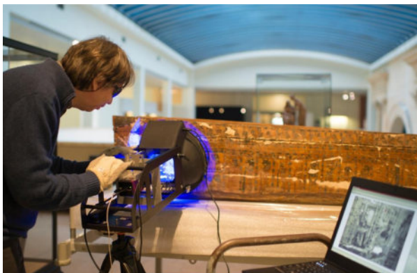
Figure 1. Example of a scanning session with a multispectral PLD at the Royal Museum for Arts and History (© KMG-MRAH)
