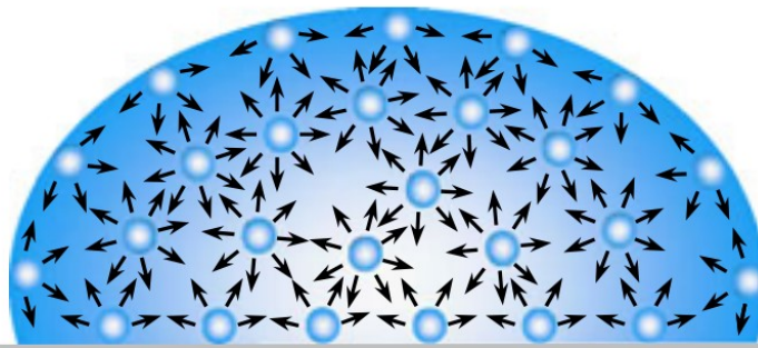
Figure 13 Representation of the surface tension caused by the unbalanced forces of liquid molecules at the surface. Reproduced from [64]
