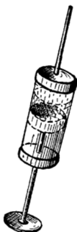
Picture 13.1. The syringe for determination of CO 2 concentration.
