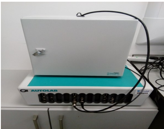
Fig. 3. Laboratory based tabletop potentiostat, the Autolab PGSTAT302N.
